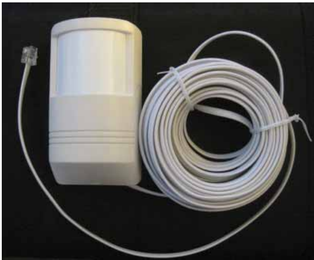
Active devices, such as PIR motion sensors and beam sensors that typically run on 12 volts DC power, require a four-wire hookup—two for power and ground, and two for the contact closure.
