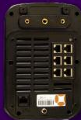
Rear view of TT Sensor (Actual size approx 20cm x 14cm)
