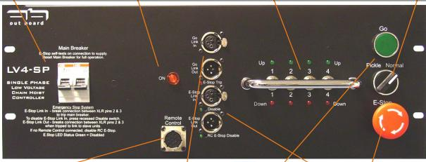
Remote operation of the LV4SP is available using the optional RC4 remote control handset, which provides Up/Down switches for motor direction, GO and E-Stop. The RC4 handset is connected to the LV4SP via a detachable multicore cable. Two LV4SP's can be run from one RC8 eight-channel handset via an RC Handset Splitter. Programmable control systems such as the IBEX PHC+ can also connect to this Remote Control socket to automate the LV4SP.
