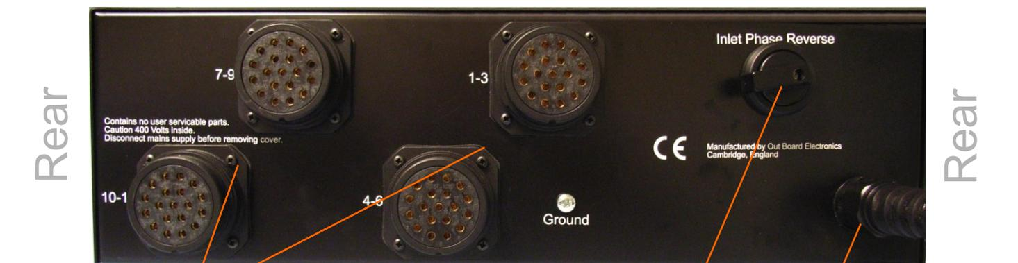
Connections to hoists are arranged on four female 19-way Socapex connectors, in groups of three channels of Up/Down control and 3-phase power/earth on each.
